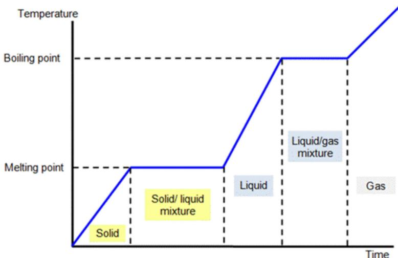
The graph above shows that the temperature of a substance does **not** change during **changes of states** instead remains constant. This is because of the energy going into the material is **overcoming** the intermolecular forces between the particles when the substance is **heated**, and is released when molecules **reform** due to the intermolecular forces when the substance is **cooled**,
